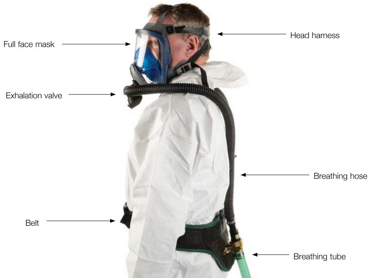
Figure 15 Fresh air hose (FAH) breathing apparatus
