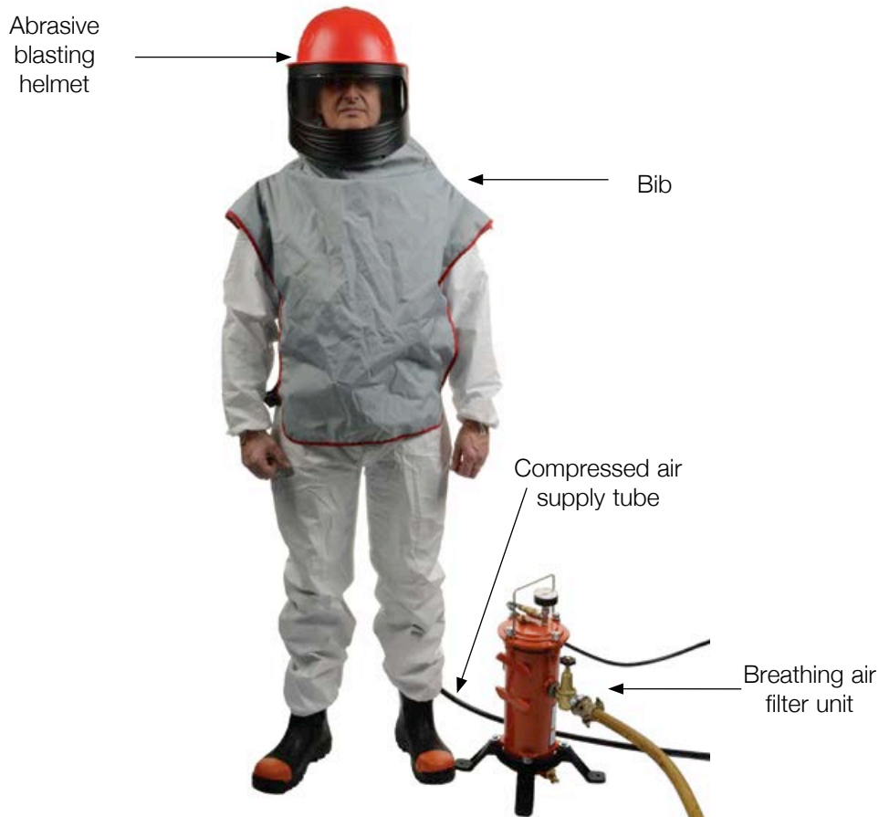
Figure 19 Constant flow airline breathing apparatus with hoods/helmets
