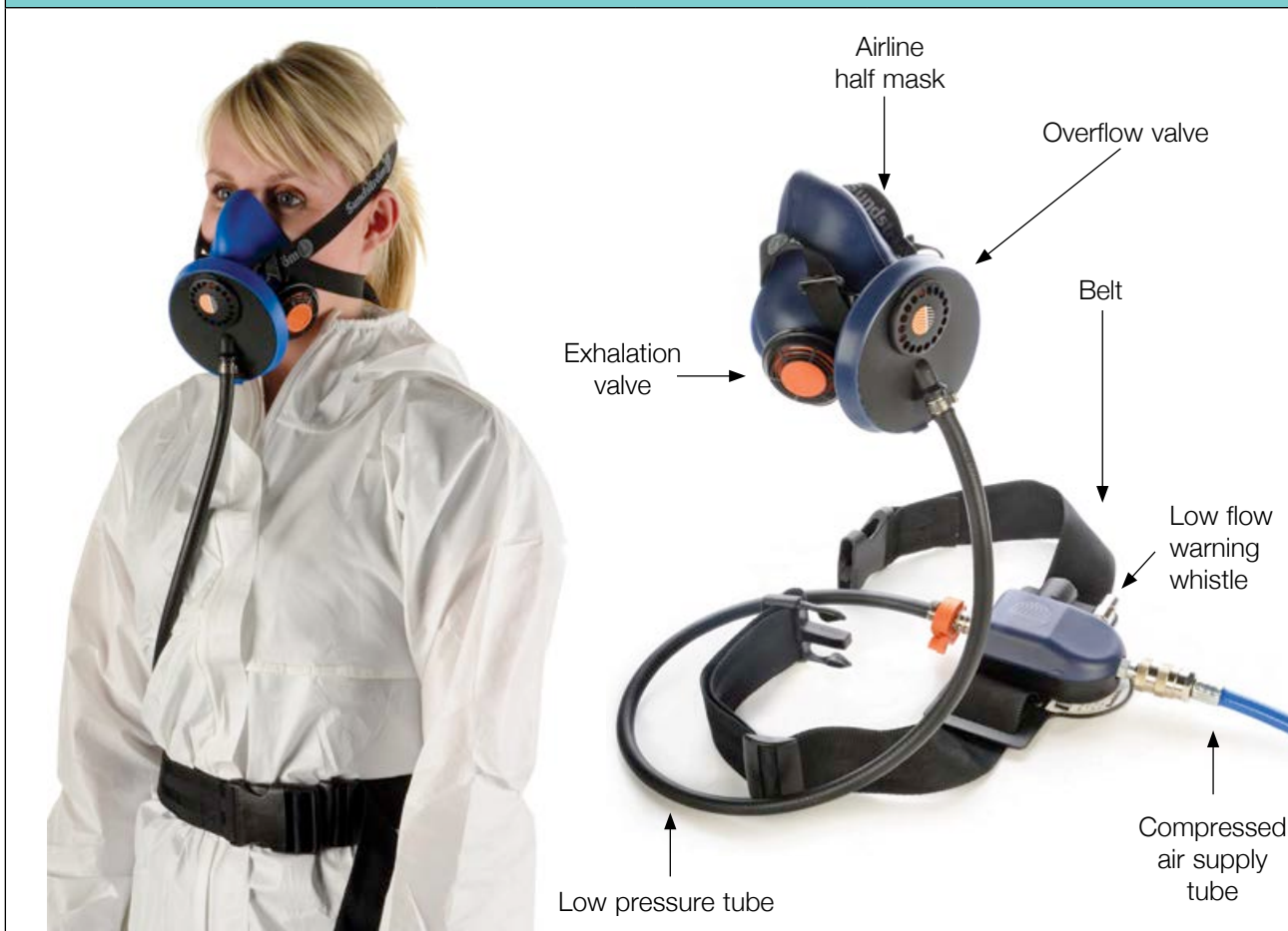
Figure 16 Constant flow airline breathing apparatus with a mask – light duty
